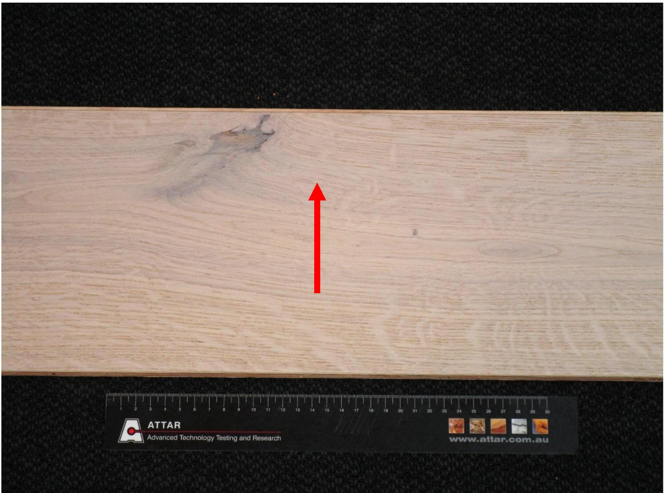
**Figure 1:** De Marque Engineered Oak 120, 190, 240 & 300 mm stair tread and nosing. Arrow indicates direction of testing.
