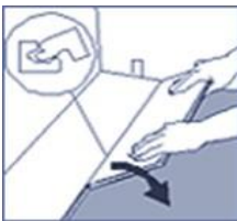
Fig 3. Tilt / Angle the plank down. During the angle process make sure the planks are tight against each other. Afterwards press down or slightly tap down at the short end or long edge of the installed plank till its flat. No major force is or required, use a tapping block or piece of softwood to avoid edge damage.
