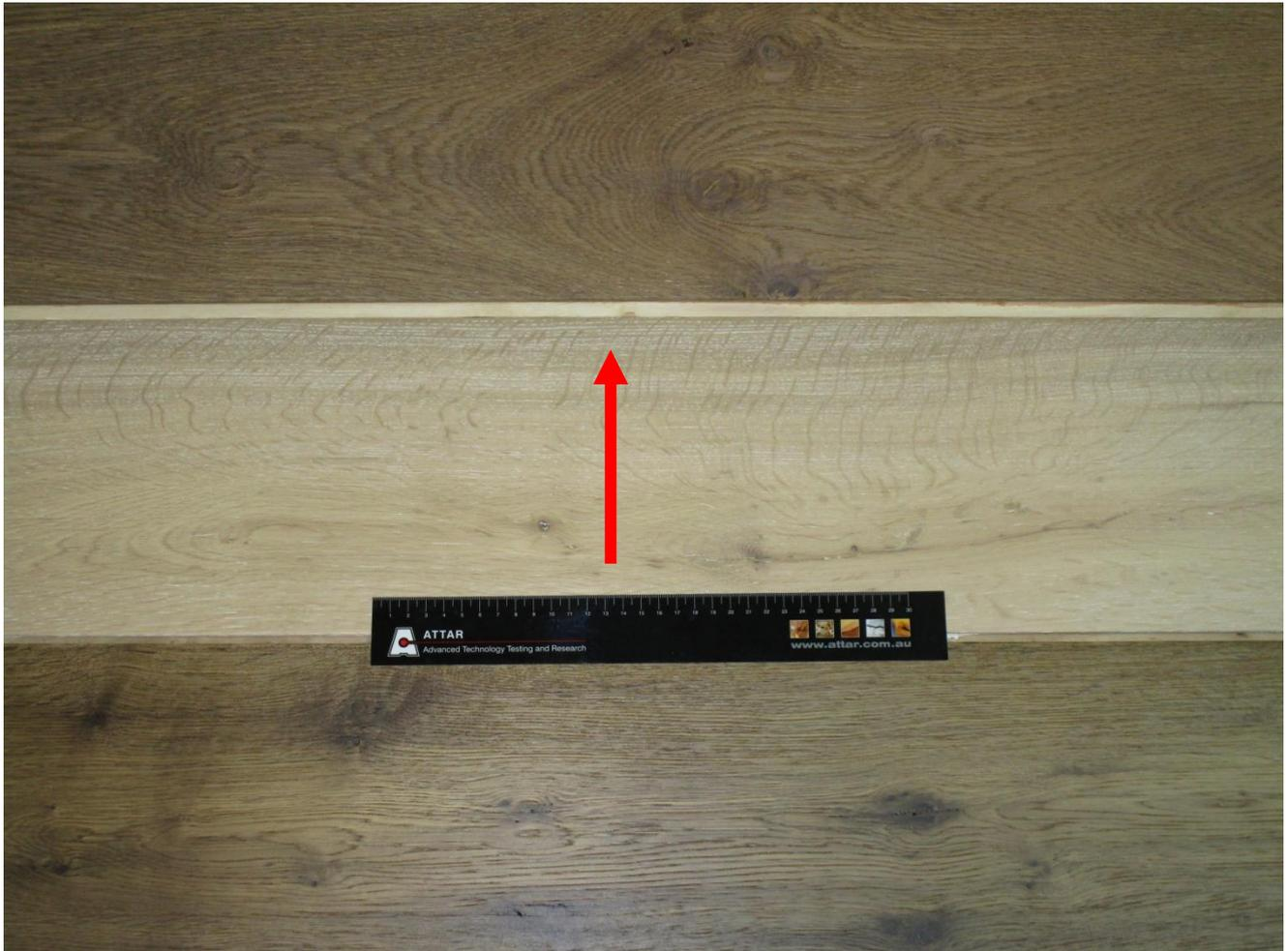
**Figure 1:** Prestige Engineered Oak 190mm & 220mm stair tread and nosing. Arrow indicates direction of testing.
