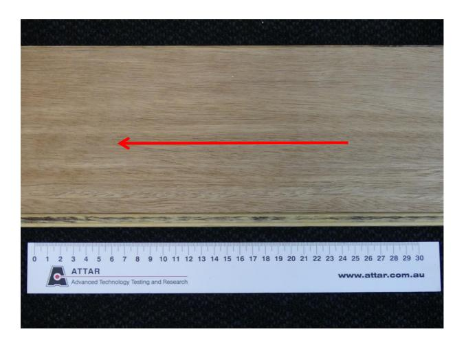
Figure 1: Eng Aust. Species brushed matte plank Arrow indicates direction of testing
